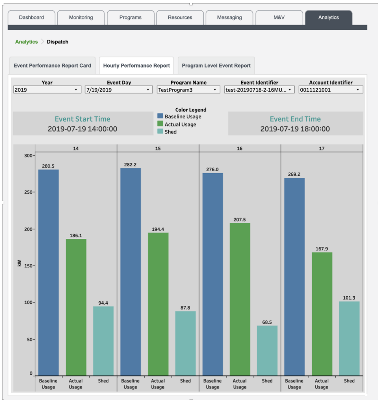
Figure 18: Example analytics toolkit showing load shed performance of an event by the hour.
